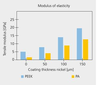
Rising modulus of elasticity for coated polymers (PEEK and PA) with increasing coating thickness.
