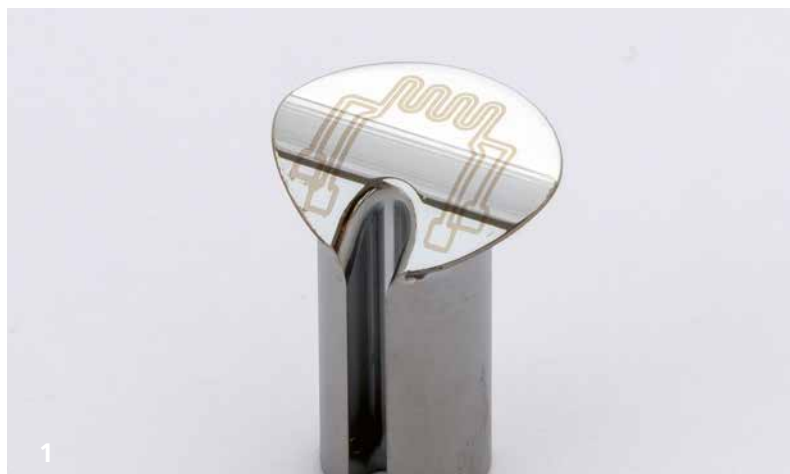
Sensor insert coated with thin-film sensors.
