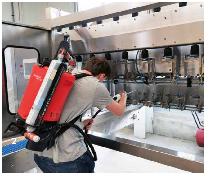
Mobile system for the spraying of ozonated water for the surface disinfection of an asparagus-peeling machine.
