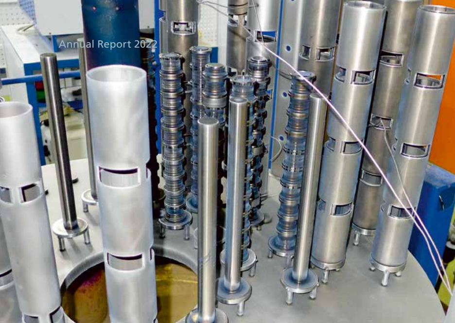
In realistic industrial setups, the treatability of bearing rings was investigated in batch processes. The batching of individual bearing rings was performed in corresponding fractions.
