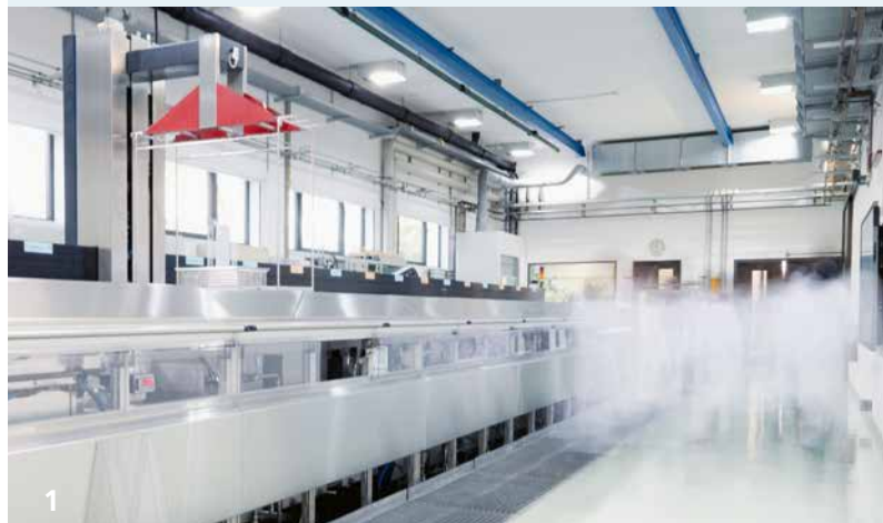
1 Visit to the multi-chamber system for aqueous cleaning at the Fraunhofer IST.
