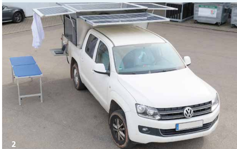
2 Prototype of the mobile supply unit mounted on a commercial pickup truck. © Fraunhofer ISE; Joachim Went
