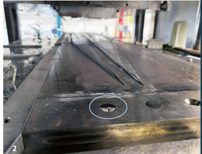
Flat-die tool with integrated sensor insert. 1
