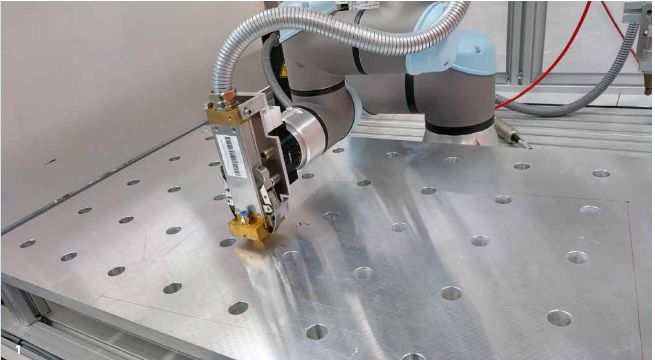
Atmospheric pressure plasma treatment system for medium-sized 3D components (< 50 cm x 50 cm x 80 cm) with robot-guided plasma nozzle.
