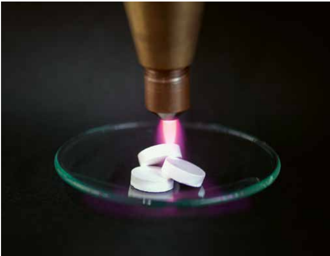
Functionalization of active ingredients and excipients by means of plasma processes for the optimized production of individualized pharmaceutical products.
