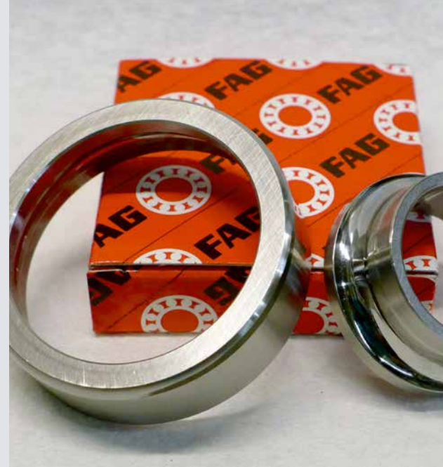
Treatment of an outer ring tower by means of low-temperature plasma nitriding.
