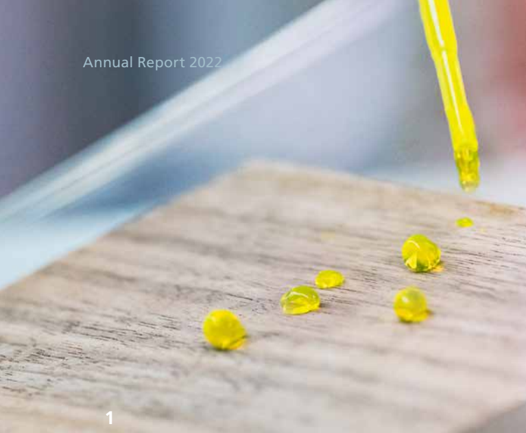
Dirt-repellent coating on a wood veneer.
