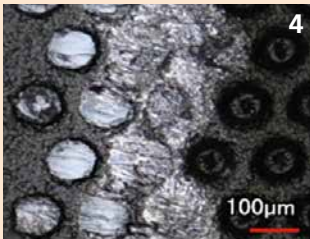
Textured chip surface with diamond and run-in layer following turning of AlSi17.
