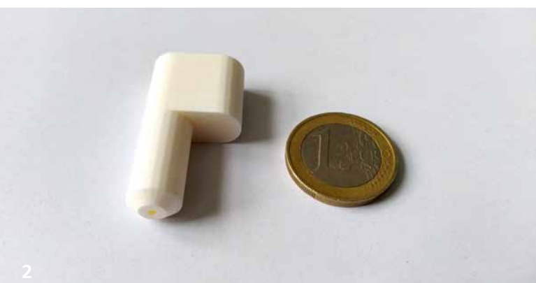
Plasma nozzle made from \text{Al}_2\text{O}_3 ceramic with size comparison.
