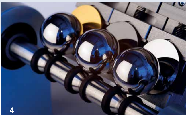
Ball-cratering device with three balls to determine precisely the wear resistance of coatings and surfaces.
