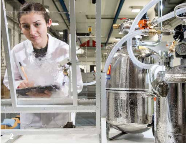
Determination of the self-cleaning effect of photocatalytically active materials and surfaces by means of the Dirt Test.
