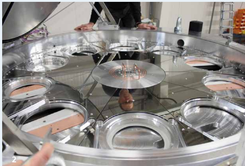
Top view of the turntable of the EOSS ® sputter system from above.
