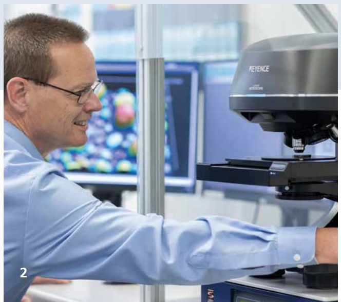
Confocal laser microscope: analysis of battery particles.
