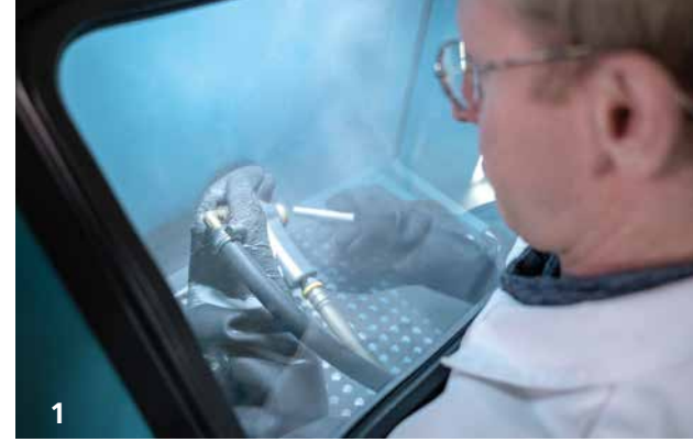
Manual blasting facility for a wide variety of blasting media.
