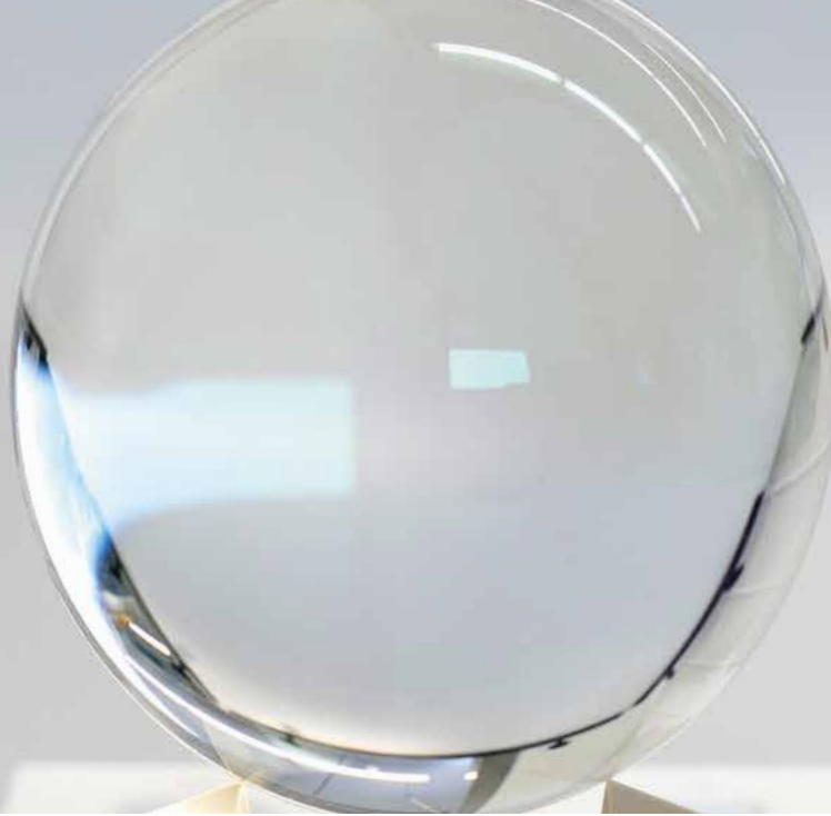
Antireflective layer system on 3D object produced by atomic layer deposition (ALD).
