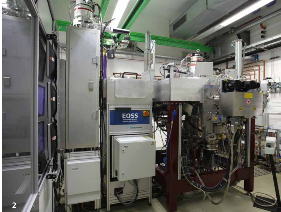
2 With the EOSS® system, state of the art high-precision coatings can be produced.
