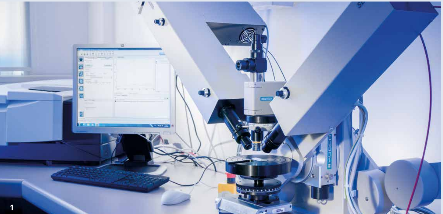
Ellipsometry for determination of thicknesses and dispersions of layers using Sentech SE 850 (SENresearch).
