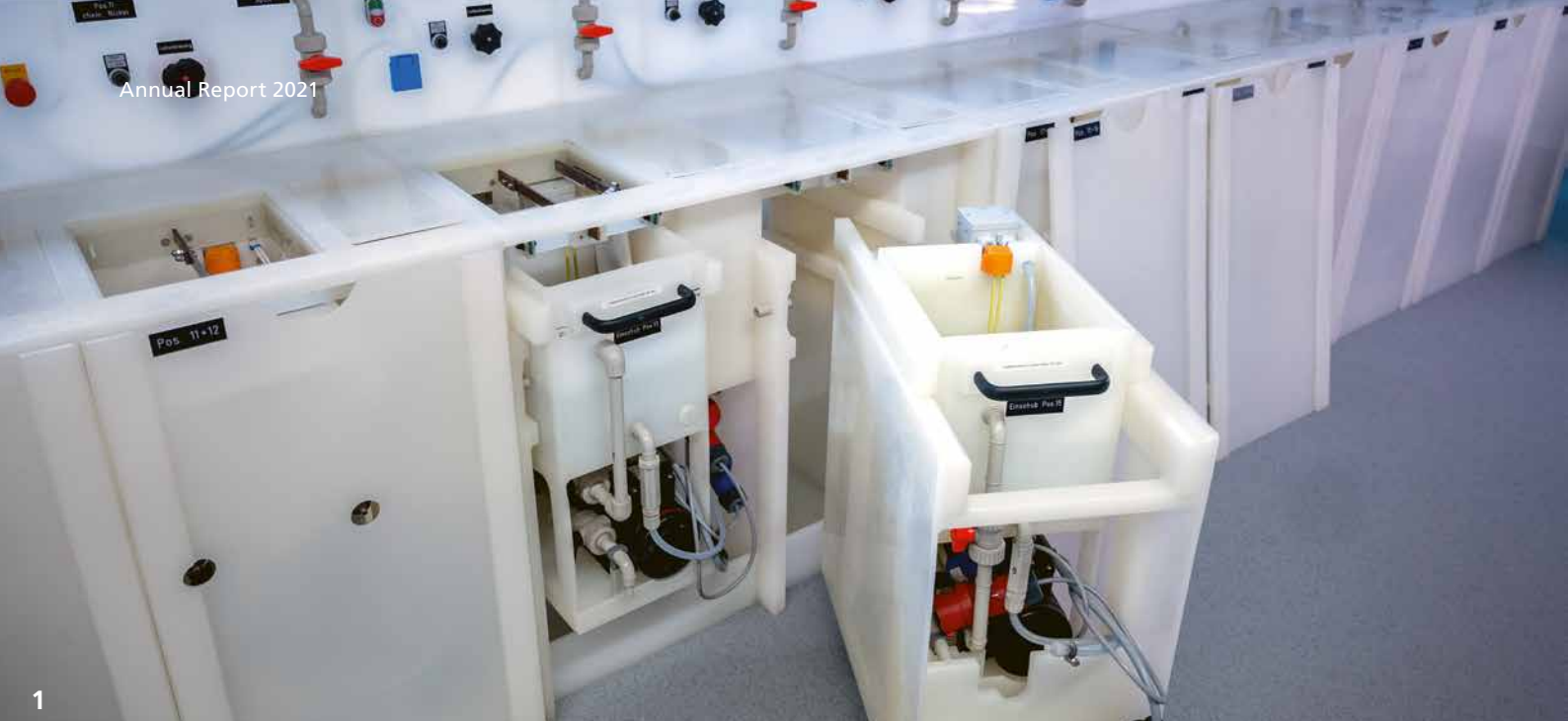
Modular, process-controlled electroplating plant on a 20-liter scale with integrated bath analysis and automated post-dosing.
