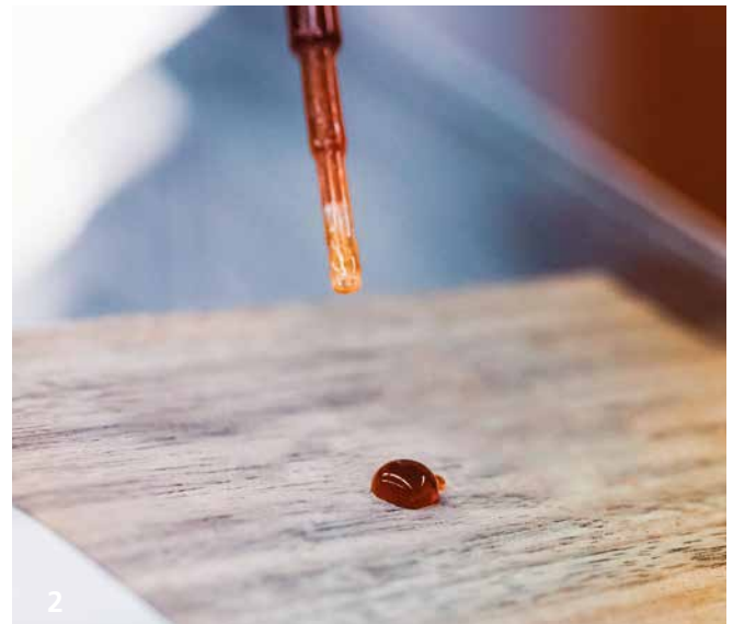
Veneer sustainably coated by means of atmospheric-pressure plasma process.
