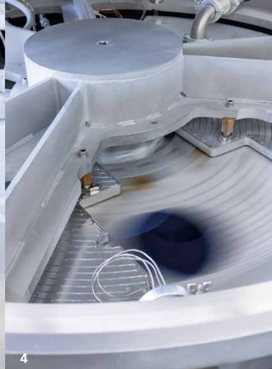
Local atomic layer deposition: View of the rotating turntable below the heating block in the hybrid area.
