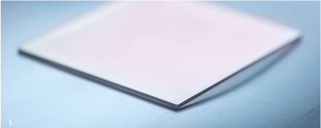
Diamond-coated quartz glass with very homogeneous coating pattern.
