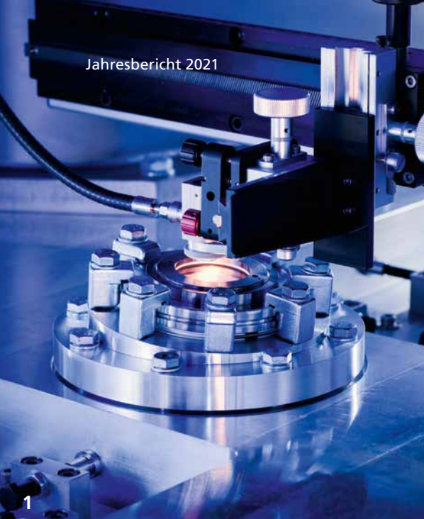
1 Optical broadband monitoring system MOCCA+®.
