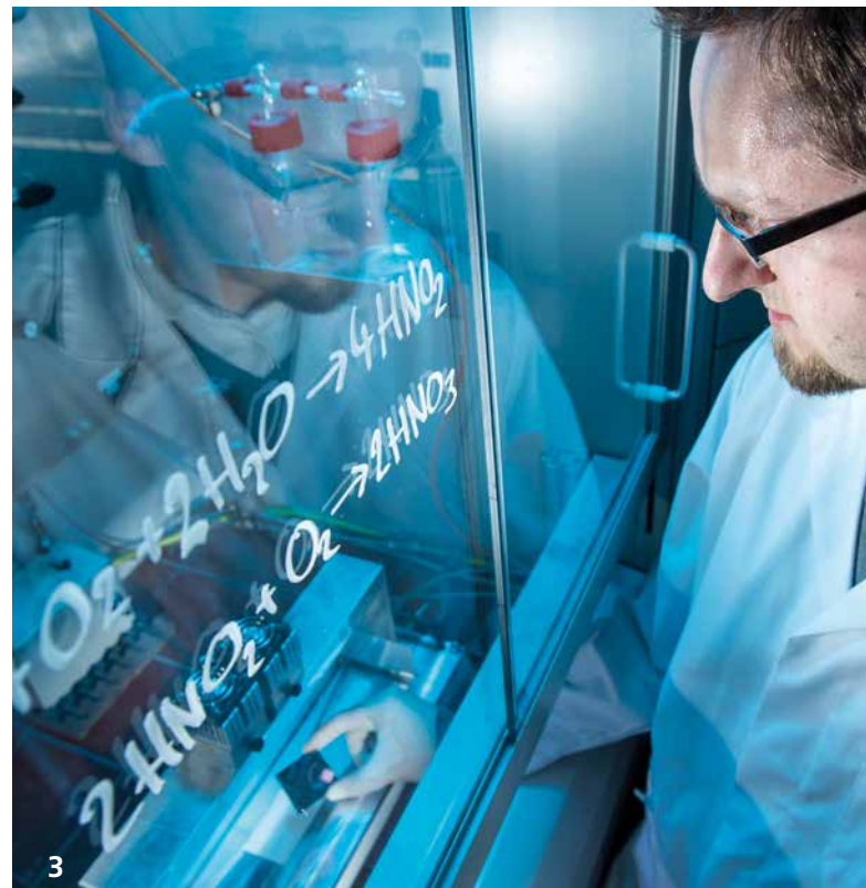
Determination of the air-purification effect of photocatalytically active materials and surfaces - degradation of nitrogen oxide.
