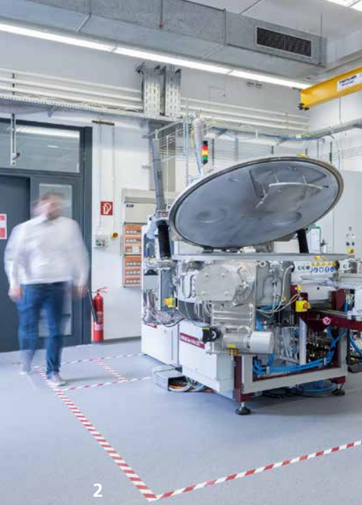
FHR Star 400x300 SALD coating system for thermal local atomic layer deposition.
